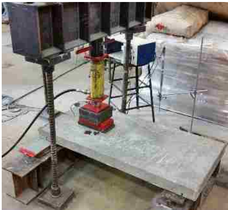
Figure 6.43. Panel SUN3 test setup
