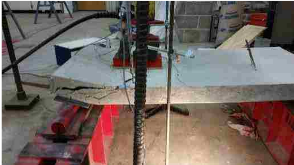
Figure 6.35. Diagonal tension failure on panel SCC3
