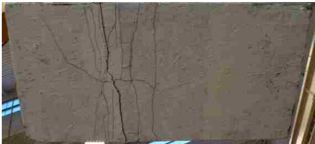
Figure 6.40. Crack pattern formation at the tension face of panel SUC3
