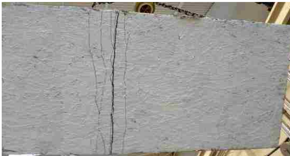
Figure 6.56. Crack pattern formation at the tension face of panel SUN2
