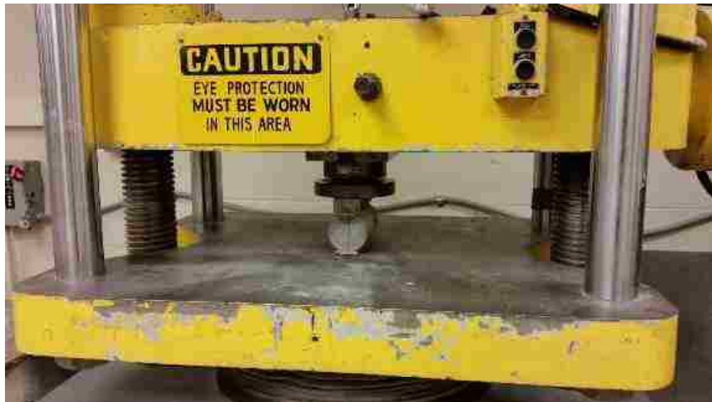
Figure 5.5. Split tensile strength test setup
