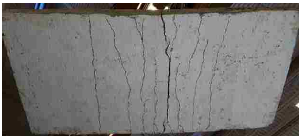
Figure 6.16. Crack pattern formation at the tension face of panel FUW3
